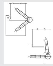
Load capacity with 2 hinges  $80\ \mbox{kg}$
