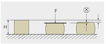
**High weather tightness** given by adapted inner diameter of the sealing washer with the fastener geometry.
