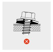
Fastener with sealing washer can only be set correctly by using setting tools equipped with depth locator. Setting with a depth locator results in a uniform setting depth for all fastener.
