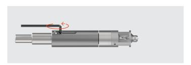
• Completely loosen the pin with a hex wrench SW2.5
