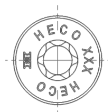
Head markings for d = 7.0 bis 10.0 mm all head types Head types without lettering possible.
